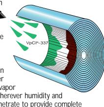
phase action migrates wherever humidity and corrosive agents can penetrate to provide complete corrosion protection. It protects external surfaces as well as internal layers of coils or sheets.
